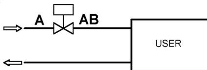
Fig. 1 Variable flow control to the user.
